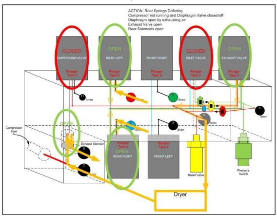
The compressor will not/should not run when the air springs are deflating.
