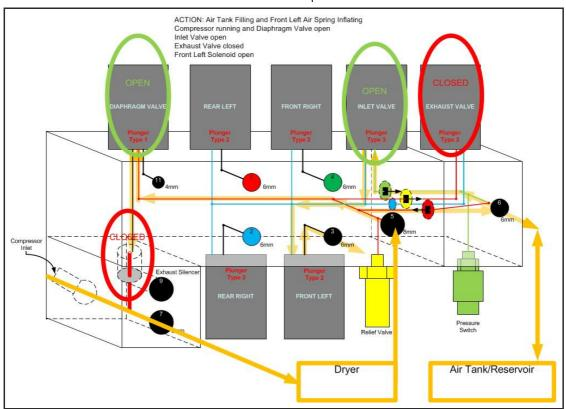
When the compressor is running, the compressor relay RL20 also operates the diaphragm valve solenoid which forces air down over the top of the diaphragm and holds it closed. This directs all incoming air from the compressor through the dryer via port 7 and back in to the valve block at port 5. With the inlet valve and exhaust valve closed, no air can flow to/from the air spring solenoids, forcing all air to the tank via port 6.
