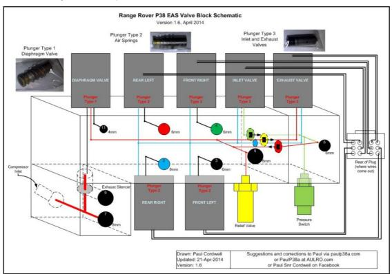
How the Valve Block Operates
